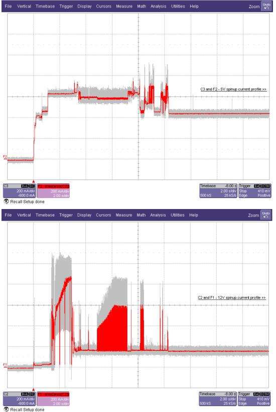
The +12V (top) and +5V (bottom) current profiles for the Constellation drives are shown below.
